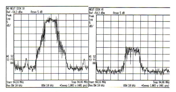
**Figure 7:** Typical spectrum analyzer traces centering at 94.16 MHz. Peak heights are related to the intensity of cellular phones radiation. Left trace is a recording from a normal cellular phone and the right trace is recorded from the same cellular phone with the shielding device attached.
